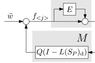
Fig. 2. Feedforward propagation structure operating in the trial domain for studying the effect of interaction on ILC. Note that  $I + E$  is invariant to  $Q$ , and measures on  $I + E$  can be developed to design for convergence.
