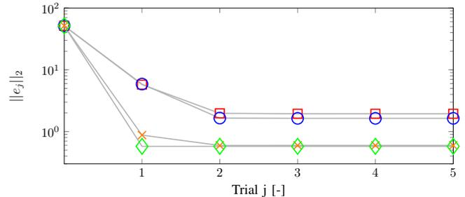
Fig. 5. Benefits of designing multivariable ILC for interaction: the centralized  $L$ -filter designs (—×—, —◇—) outperform the decentralized designs (—□—, —○—), which require robustness to both modeling errors and ignored interaction. Also, through independent  $Q$ -filter designs (—○—), ignored interaction is addressed appropriately, which potentially improves performance compared to conservative  $Q$ -filter design (—□—) for *worst-case* interaction.
