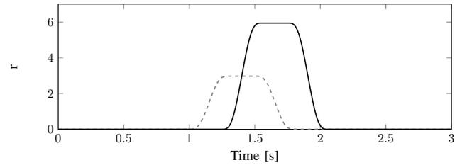
Fig. 4. Fourth order reference signals for input 1 (---) and input 2 (—).
