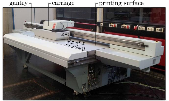
Fig. 5. Océ Arizona 550 GT at the CST Motion laboratory, Eindhoven University of Technology. The  $x$  and  $\varphi$  positions of the carriage are considered for control.
