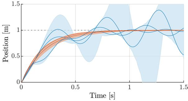
Fig. 7. Unit step response of the closed-loop system evaluated at randomly selected frozen operating points  $\{p^{(\tau)}\} \in \mathbb{P}$ , using the 2nd order LTI and LPV FIR controllers in blue and orange lines, respectively. The LTI controller that is used is equal to the one for  $p = 0$  given in Table 2. The blue and orange shaded areas indicate the regions that cover all trajectories for frozen  $\{p^{(\tau)}\} \in \mathbb{P}$  for the LTI and LPV controllers, respectively.
