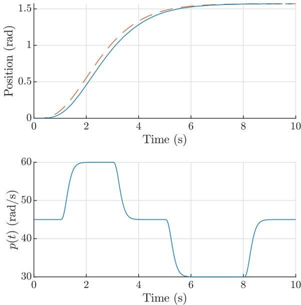
Fig. 8. Reference tracking of the gyroscope using the 2nd order LPV FIR controller. Angular position of gimbal A in blue and the reference in dashed orange (upper plot). Scheduling variable  $p(kT_s) = \dot{q}_{1,*}(kT_s)$  (bottom plot).
