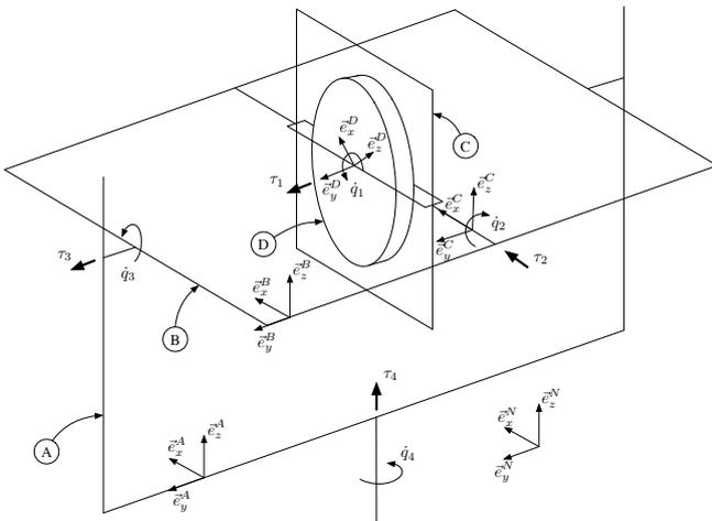
Fig. 1. Schematic overview of the 3-DOF gyroscope.
