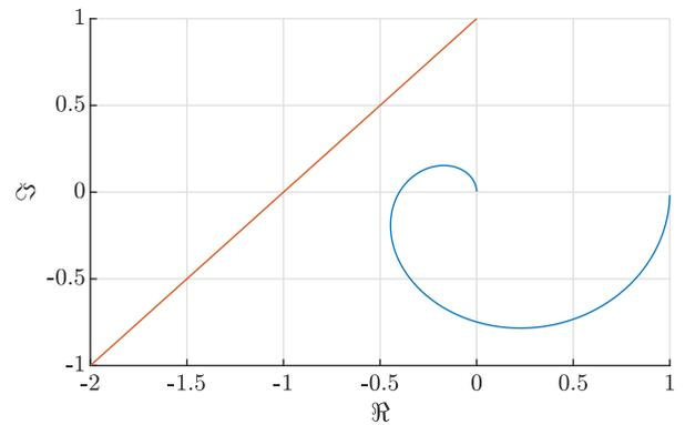
Fig. 5. Graphical interpretation of the simplified Nyquist stability criterion. The line (orange) restricts the Nyquist curve to lie to the right of the critical point  $(-1, 0i)$ . The Nyquist curve  $L_p(e^{i\omega}, \theta)$  (blue) is shown for a constant operating condition  $p$  and fixed  $\theta$ .
