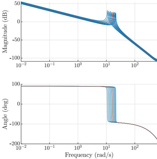
Fig. 2. Magnitude and phase plots of the FRF data of the gyroscope obtained at the operating points  $\{p^{(\tau)}\}_{\tau=1}^{N_p} \subset [-1, 1]$  (rad/s) are plotted in blue and the nominal FRF at  $p = 0$  (corresponding to  $\dot{q}_{1,*} = 45$  (rad/s)) is plotted in orange.
