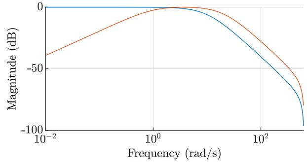
Fig. 6. Magnitude plot of the model-matching filter  $M(e^{i\omega})$  in blue and the weighting filter  $W(e^{i\omega})$  in orange.
