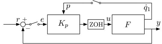
Fig. 4. Interpretation of the closed-loop implementation of the LPV controller with the plant. Here  $K_p$  is the discrete-time LPV controller scheduled by a time-varying  $p$  and  $F$  represents the continuous-time nonlinear system (1) where  $p$  is measured.
