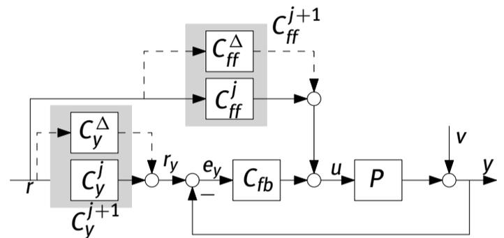
Control Configuration for optimization-based feedforward
