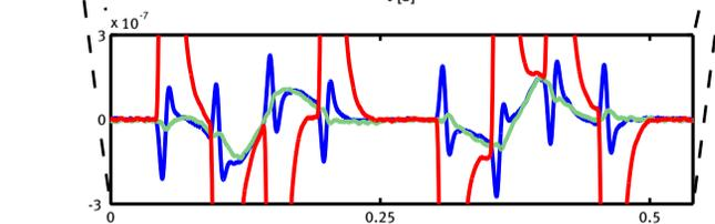
Servo error as function of tasks - 1<sup>th</sup> (red), 2<sup>nd</sup> (blue) and 3<sup>th</sup> (green) task
