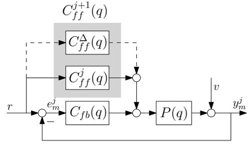
Fig. 2: The feedforward controller  $C_{ff}^{j+1}$  is determined based on the reference  $r$ , and measured signals  $y_m^j$  and  $e_m^j$  in the  $j^{\text{th}}$  task.
