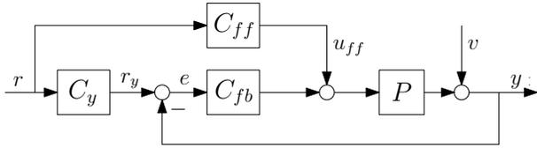
Fig. 1: Two degree-of-freedom control configuration.
