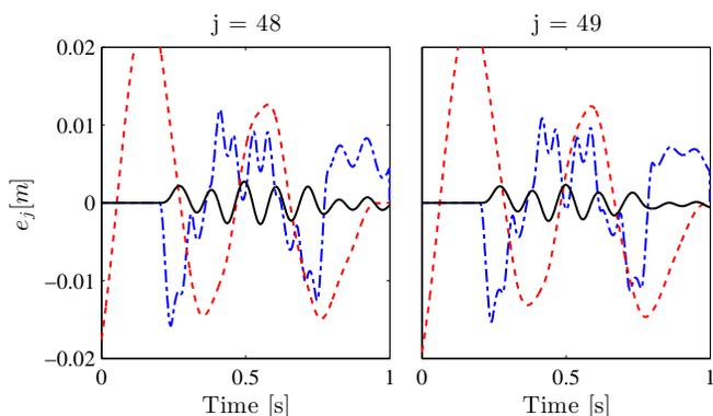
Fig. 5. Tracking errors  $e_{48}$  (before reference change) and  $e_{49}$  (after reference change): proposed (black solid), FIR (blue dash-dotted), extended FIR (red dashed).
