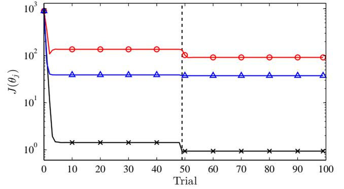
Fig. 3. Cost function  $J(\theta_j)$ , proposed ( $\times$ ), extended FIR ( $\circ$ ), FIR ( $\triangle$ ), reference change from  $r_1$  to  $r_2$  (black dashed).
