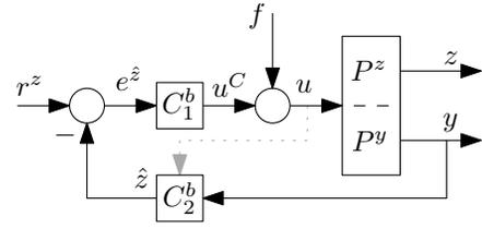
Fig. 4. Different 2-DOF feedback control structure for inferential control.
