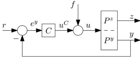
Fig. 2. Conventional feedback control structure with feedforward  $f$ .
