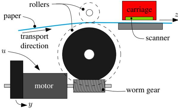
Fig. 1. Medium positioning drive: the motor is driven with voltage  $u$ , the rotor position  $y$  is measured using an optical encoder, the paper is transported by the rollers and the paper position  $z$  is measured using the scanner inside the carriage.
