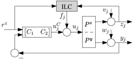
Fig. 6. Unifying 2-DOF feedback control structure with ILC for inferential control.
