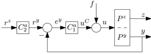
Fig. 3. 2-DOF feedback control structure for inferential control.
