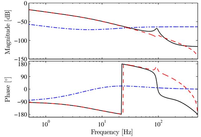
Fig. 8. Models  $P^z$  (solid black),  $P^y$  (dashed red), and 1-DOF feedback controller  $C \cdot 10^{-6}$  (dashed-dotted blue).
