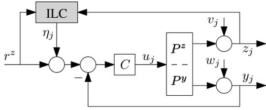
Fig. 7. Common 1-DOF feedback control structure with ILC for inferential control.
