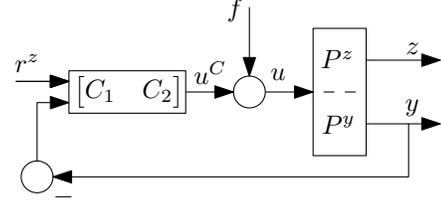
Fig. 5. Unifying 2-DOF feedback control structure for inferential control.
