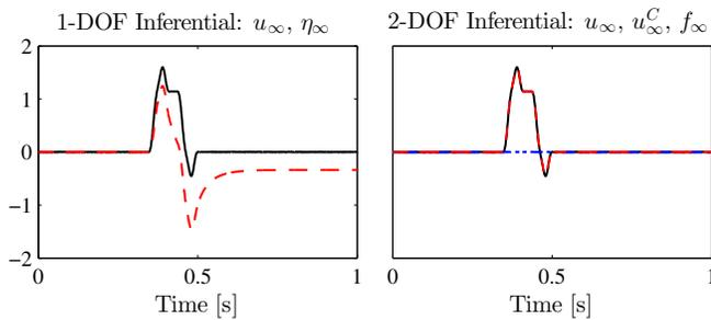
Fig. 10. Left: converged command signals  $u_\infty$  (solid black) and  $\eta_\infty \cdot 300$  (dashed red) for the inferential 1-DOF structure. Right: converged command signals  $u_\infty$  (solid black),  $f_\infty$  (dashed red), and  $u_\infty^C$  (dashed-dotted blue) for the inferential 2-DOF structure.
