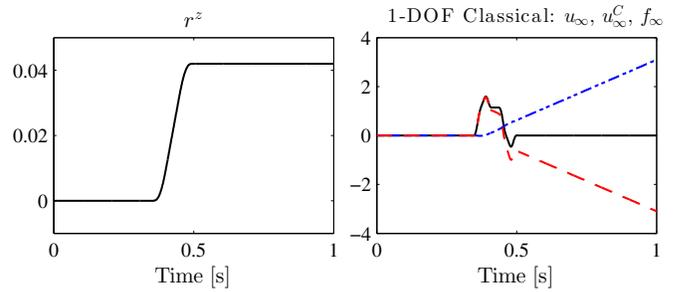
Fig. 9. Left: reference  $r^z$  (solid black). Right: converged command signals  $u_\infty$  (solid black),  $f_\infty$  (dashed red), and  $u_\infty^C$  (dashed-dotted blue) for the classical non-inferential 1-DOF structure, revealing the conflicting control objectives.
