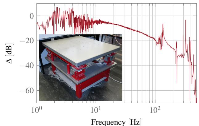
Figure 1: Measured  $\Delta$  of an AVIS
