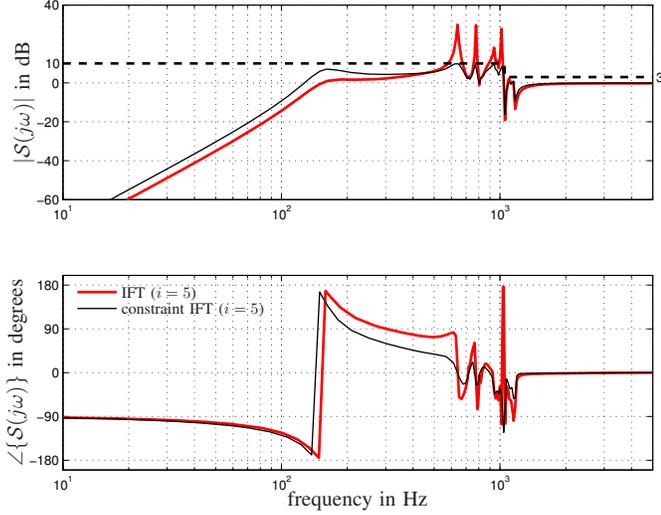
Fig. 8. Bode diagrams of the sensitivity function  $S$  based on simulated data with IFT ( $i = 5$ ), i.e., no constraints, and with constraint IFT ( $i = 5$ );  $S_b = 9.5$  dB on the interval  $f \in [0 \ 1.05]$  kHz and 2.5 dB on the interval  $f \in [1.05 \ 5]$  kHz,  $\alpha = 10 \text{ nm}^2$ ,  $\gamma_0 = 1$ ,  $\epsilon = 0.5$  dB.
