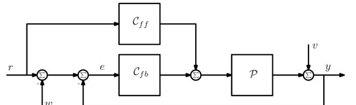
Fig. 2. Block diagram of the simplified wafer stage motion control context.
