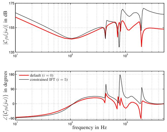
Fig. 6. Bode diagrams of the controllers before ( $i = 0$ ) and after ( $i = 5$ ) optimization.
