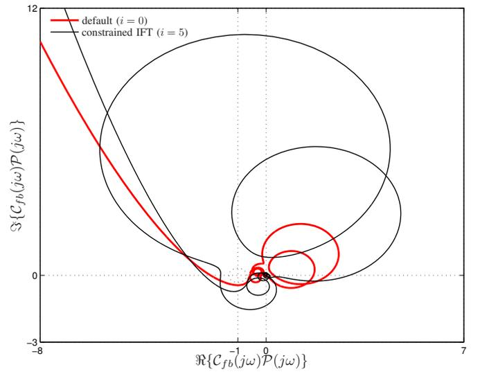
Fig. 9. Nyquist plots of the open-loop frequency response functions before ( $i = 0$ ) and after ( $i = 5$ ) optimization.
