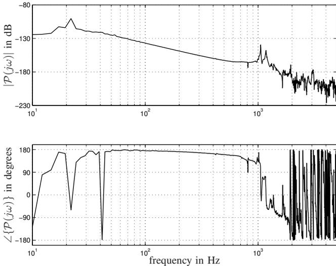
Fig. 3. Bode diagram of the short-stroke wafer stage plant  $\mathcal{P}$  in  $y$ -direction with measured data.
