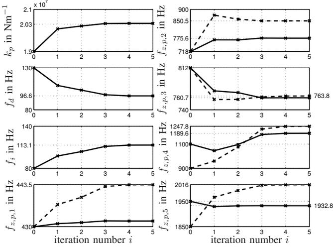
Fig. 5. Measured parameter convergence diagram; for the notch filters  $\mathcal{N}_i$  convergence of the zero frequencies  $f_{z,i} = \omega_{z,i}/2\pi$  is indicated by the solid curves while convergence of the pole frequencies  $f_{p,i} = \omega_{p,i}/2\pi$  is indicated by the dashed curves;  $\gamma_0 = 1$ ,  $\epsilon = 0.5$  dB.
