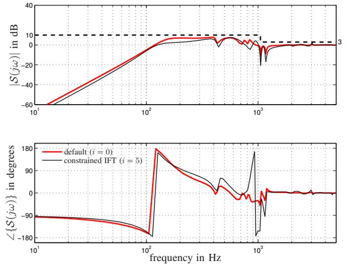
Fig. 7. Bode diagrams of the sensitivity function  $S$  based on measured data before ( $i = 0$ ) and after ( $i = 5$ ) constraint IFT optimization;  $S_b = 9.5$  dB on the interval  $f \in [0 \ 1.05]$  kHz and 2.5 dB on the interval  $f \in [1.05 \ 5]$  kHz,  $\alpha = 10$  nm<sup>2</sup>,  $\gamma_0 = 1$ ,  $\epsilon = 0.5$  dB.
