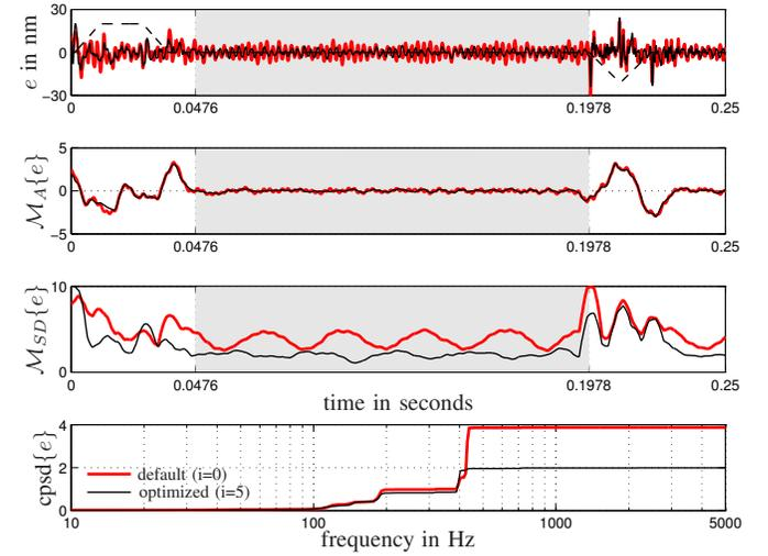
Fig. 10. Time-series representation of experimental data at iteration  $i = 0$  and iteration  $i = 5$  together with the results from cumulative power spectral density analysis; the scaled acceleration set-point profile is indicated with dashed lines; the scanning performance window is indicated in grey.
