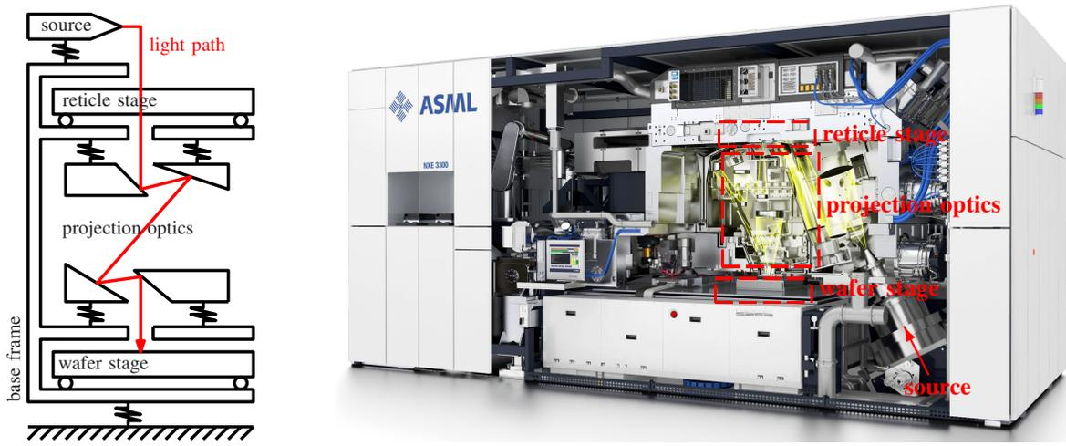
Fig. 1. Schematics and artist impression of a wafer scanner.
