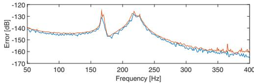
Fig. 2: Estimation errors of the estimated plant  $\hat{G}$  with respect to the true plant  $G_{LPV}$ , averaged over all  $\theta$ ; the traditional LPM as in [35] (red), and the proposed 2D-LPM (blue).
