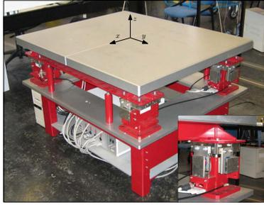
Fig. 1. Photograph of the experimental AVIS setup. The rotation around the  $x$ -axis is denoted by  $\phi$ .
