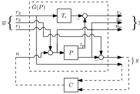
Fig. 3. Recasting the setup of Figure 2 into the standard plant configuration.
