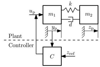
Fig. 1. Inferential servo control.
