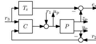
Fig. 2. Unweighted exogenous inputs and outputs.
