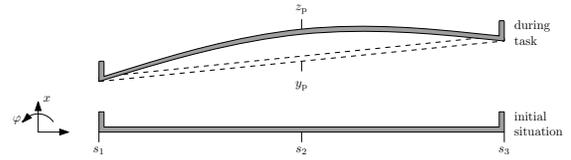
Fig. 2. Schematic top view illustration of flexible beam setup.
