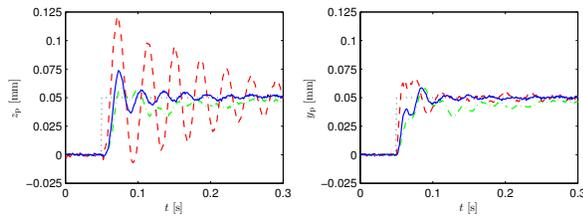
Fig. 8. Experimental step responses using robust inferential controller  $C^{\text{RP9}}$  (solid), robust 4-block controller  $C^{\text{RP4}}$  (dashed), initial controller  $C^{\text{exp}}$ .
