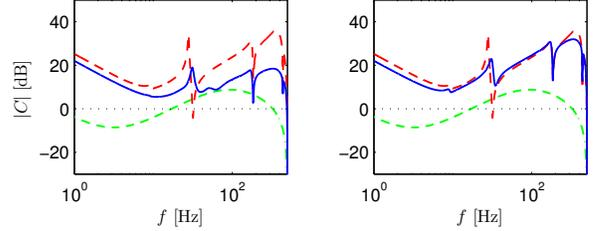
Fig. 7. Bode diagram of controller: robust inferential controller  $C^{\text{RP9}}$  (solid), robust 4-block controller  $C^{\text{RP4}}$  (dashed), initial controller  $C^{\text{exp}}$  (dash-dotted). Left:  $C_1$ , right:  $C_2$ .
