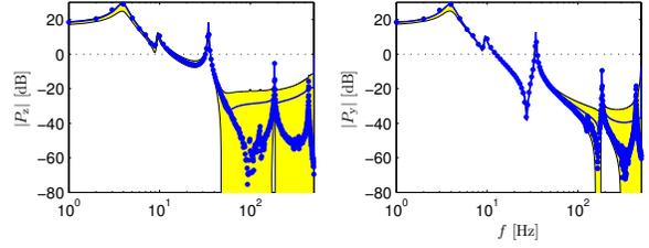
Fig. 6. Bode magnitude diagram: frequency response function corresponding to Figure 5 (dot), nominal model  $\hat{P}$  (solid), model set  $\mathcal{P}$  (shaded).
