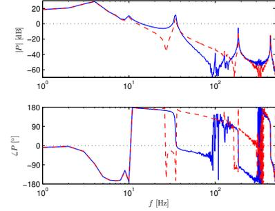
Fig. 5. Frequency response function estimate  $P_{z,o}(\omega)$  (solid),  $P_{y,o}(\omega)$  (dashed).
