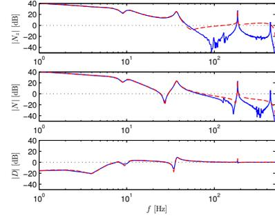
Fig. 4. Bode magnitude diagram of identified frequency response function of  $N_{z,o}, N_o, D_o$  (solid) and identified parametric model  $\hat{N}_z, \hat{N}, \hat{D}$  (dashed).
