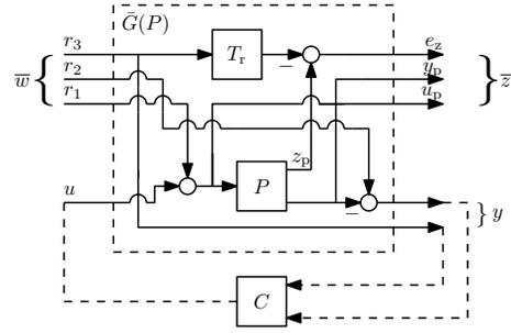
Fig. 3. Standard plant configuration for inferential control.
