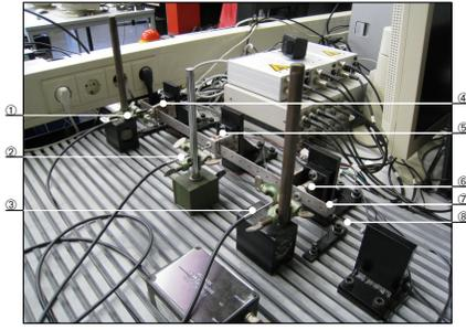
Fig. 1. Photograph of the experimental flexible beam setup, where ①: sensor  $s_1$ , ②: sensor  $s_2$ , ③: sensor  $s_3$ , ④: actuator  $a_1$ , ⑤: actuator  $a_2$ , ⑥: actuator  $a_3$ , ⑦: beam, ⑧: leaf spring.
