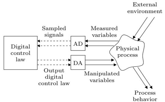
Fig. 2. Process controlled by a digital controller
