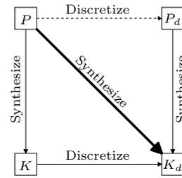
Fig. 6. Design of a digital controller for a CT plant
