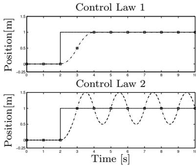
Fig. 8. Reference signal (solid), CT response  $y(t)$  (dash-dotted), DT response  $\psi(kh)$  (square)
