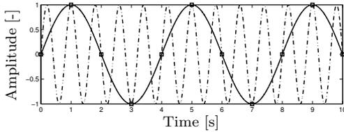
Fig. 5. Sine ( $f = 0.25$  [Hz]) (solid), sine ( $f = 1.25$  [Hz]) (dash-dotted), sampled sine (square)
