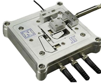
Fig. 1. Three-axis nanopositioner.
