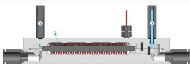
**Figure 1.** A cross-section of the Local Fluid Stream Heater used in this research, with incoming temperature sensor (1), outgoing temperature sensor (2) and heater coil (3).
