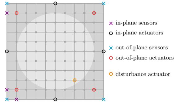
Fig. 2. Schematic top view of the experimental setup.
