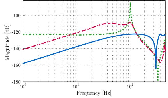
Fig. 5. Comparison of high and low gain observer. Shows the response from disturbance  $d$  to  $e_z = z - \hat{z}$  for the rigid body estimation (green, dotted), low gain observer (red, dash dotted) and high gain observer (blue, solid).
