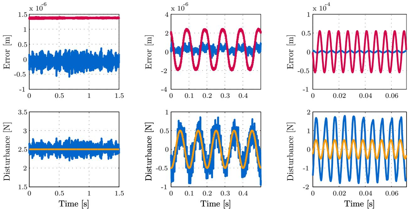
Fig. 8. Results of time domain experiments, showing the response to a constant (left), 10Hz (middle) and 140Hz (right) disturbance. The top plots show  $e_z = z - \hat{z}$  for the rigid body estimation (red) and the designed high gain observer (blue), bottom shows the applied disturbance (orange) as well as the disturbance as estimated by the observer (blue).
