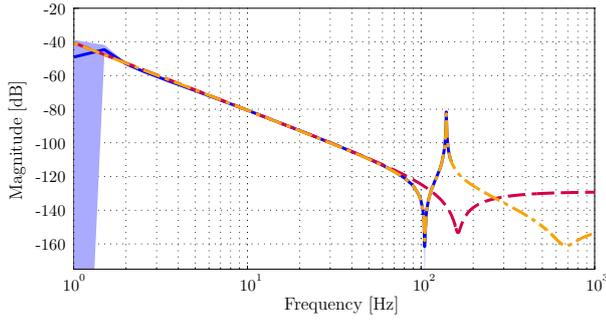
Fig. 6. Identification results for the (1,1) element, showing the identified FRF (blue, solid) with 95% confidence bound (light blue) and two identified models: one with the resonance (orange, dash dotted) and one without the resonance (red, dashed).
