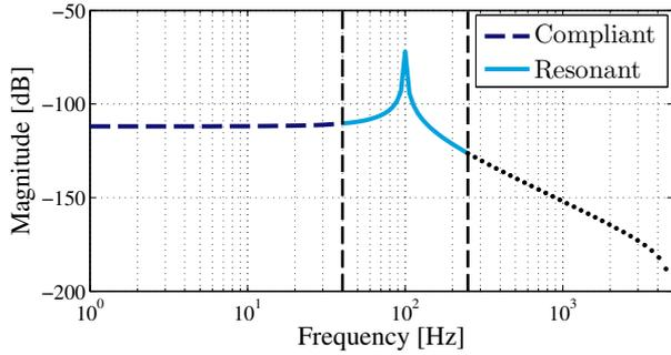
Fig. 4. Compliant and resonant behavior of a flexible mode.
