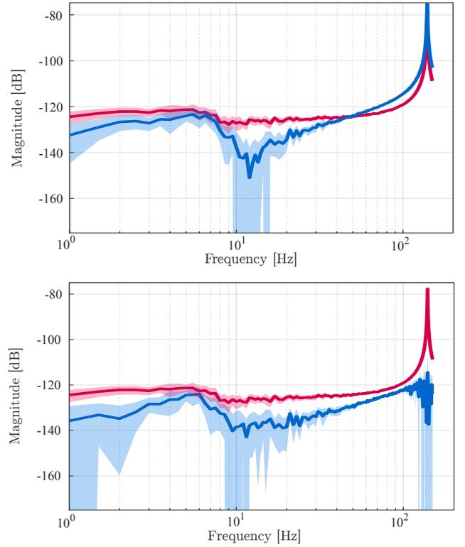
Fig. 7. Observed frequency response from  $d$  to  $e_z = z - \hat{z}$  and 95% confidence bounds for the rigid body estimation (red) and the proposed observers (blue) using the identified models without resonance (top) and with the resonance (bottom).
