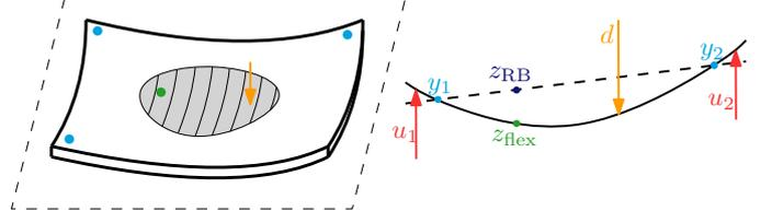
Fig. 3. Schematic deformed wafer-stage (left) and cross section (right), showing non-collocated performance location  $z$  (green), sensors  $y$  (cyan), disturbance  $d$  (orange), actuators  $u$  (red) and rigid body estimation  $\hat{z}_{\text{RB}}$  (dark blue).
