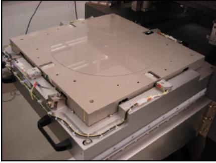
Fig. 1. The experimental setup: a prototype wafer stage.
