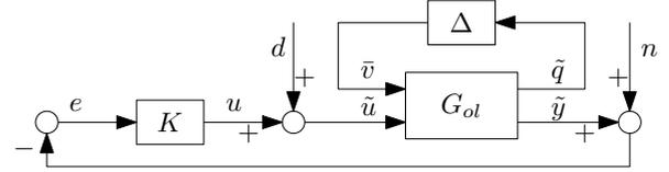
Fig. 4. Linear drill-string dynamics  $G_{ol}$  in closed loop with the controller  $K$  and including model uncertainty  $\Delta$ .
