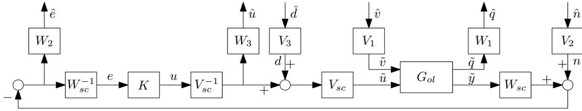
Fig. 5. Closed-loop system with weighting filters and scaling matrices.
