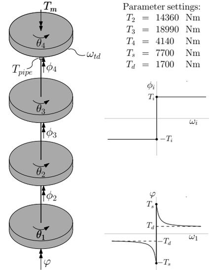
Fig. 2. 4-DOF model of the drill-string.
