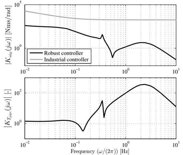
Fig. 6. Designed linear dynamic controller for the drill-string system, upper plot is the controller which uses the top drive angular velocity, the controller in the lower plot is based on the pipe torque measurement.
