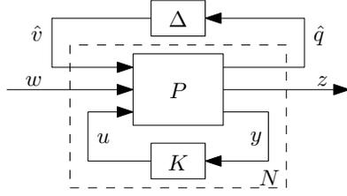
Fig. 3. Control configuration with uncertainty block  $\Delta$ .
