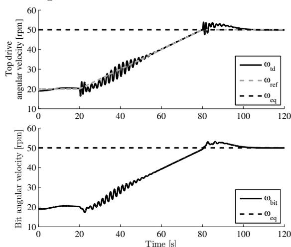
Fig. 8. Simulation result of the drill-string model with the designed output-feedback controller.
