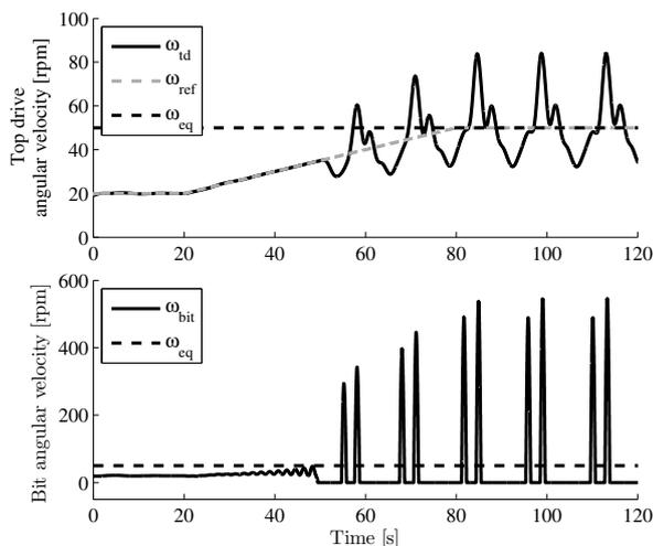
Fig. 7. Simulation result of the drill-string model with an existing industrial controller.
