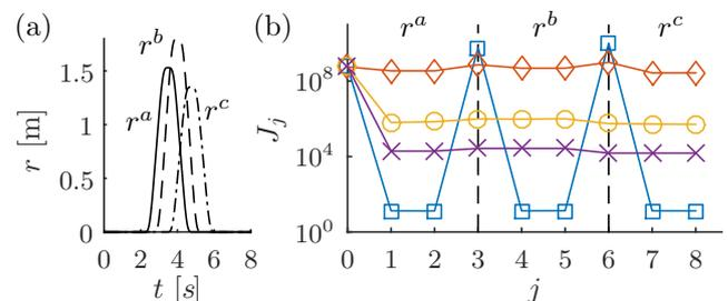
**Figure 3:** (a) trial varying reference signal; (b) performance criterion  $J_j$  for standard ILC ( $\square$ ), polynomial basis functions using the pre-existing approach ( $\diamond$ ), and rational basis functions using the proposed approach ( $\times$ ).
