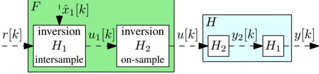
Fig. 2. The discrete-time system  $H$  is decomposed into  $H_1$  and  $H_2$ . System  $H_1$  is inverted such that there is exact state tracking of the desired state  $\hat{x}_1[k]$  every  $n_1$  samples for the purpose of intersample behavior. System  $H_2$  is inverted such that there is exact output tracking every sample for the purpose of on-sample behavior.
