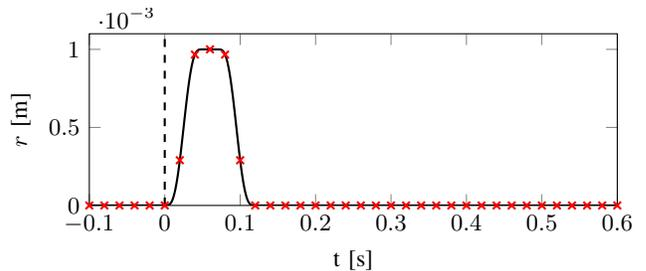
Fig. 5. The reference trajectory  $r(t)$  (—), with discretization  $r[k]$  (x). The trajectory consists of a forward and backward movement.
