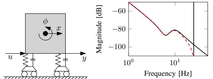
(a) The system is actuated by input force  $u$ , can translate in  $x$  direction, rotate in  $\phi$  direction, and has output position  $y$ . (b) Bode magnitude diagram of the continuous-time system  $H_c$  (—) and the discretized system  $H$  (---) from input  $u$  to output  $y$  in (a).
