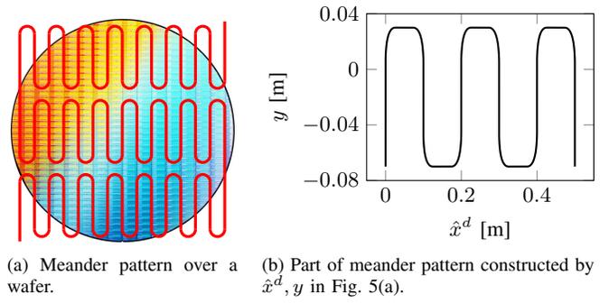
Fig. 4. The wafer is scanned by moving the wafer stage in a meander pattern.
