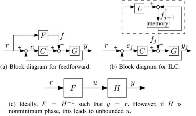
Fig. 1. Both the design of feedforward in (a) and of ILC in (b) can be captured in the structure of (c), where  $H = G$  for feedforward and  $H = SG$  for ILC.
