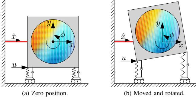
Fig. 3. Top view of wafer stage. The interferometer is fixed on the metrology frame and measures distance  $\hat{x}$  to the wafer stage which has degrees of freedom  $x, y, \phi$ . If  $\phi \neq 0$ , position  $y$  effects measurement  $\hat{x}$ .
