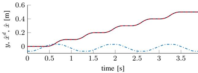
(a) Output  $\hat{x}$  with forward simulation (—) and with stable inversion (····) perfectly tracks the desired trajectory  $\hat{x}^d$  (····) for the prescribed periodic position  $y$  (- - -).
