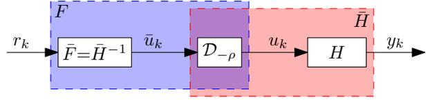
Fig. 2. Time-shifting  $u_k$  with the relative degree  $\rho$  of  $H$  allows to invert the bi-proper system  $\bar{H}$ . Signal  $u_k$  is found by applying a forward shift of  $\rho$  samples to the output  $\bar{u}_k$  of  $\bar{F} = \bar{H}^{-1}$ .
